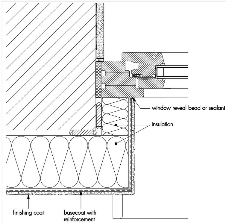
Figure 10 Window sill detail
