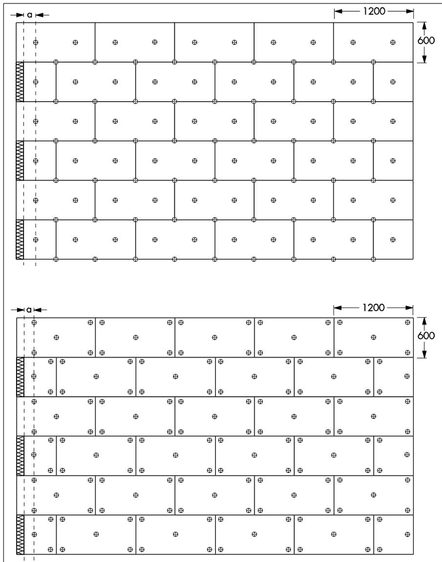
a. The minimum edge distance should be  $\geq 100$  mm.
