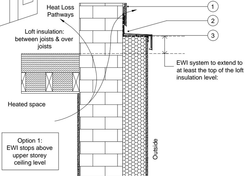
1. Render dressed down over upstand of metal using proprietary connection profile
