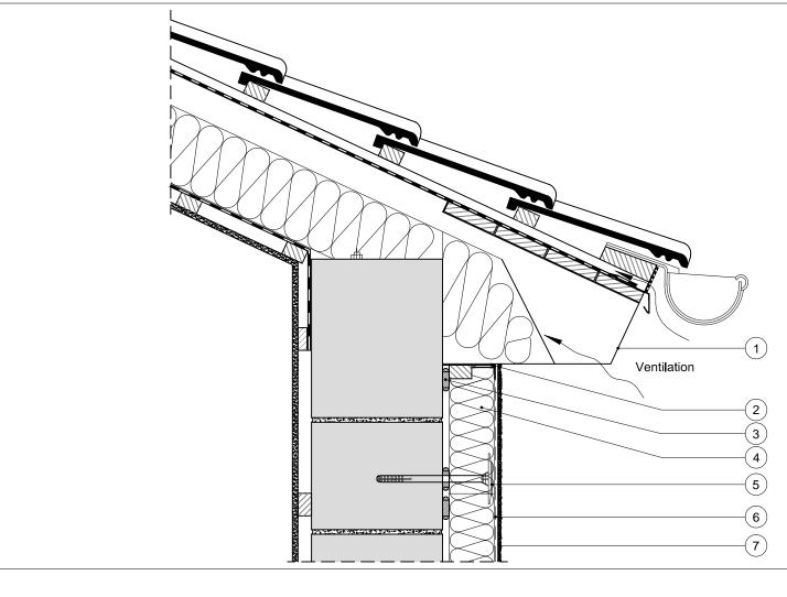
Roof profile on a sloping roof.
