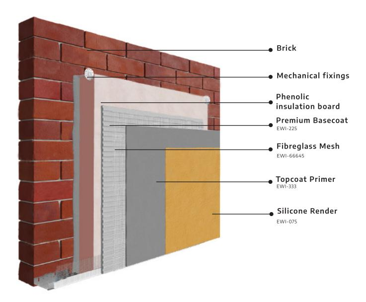
EWI-075 Silicone Render is flexible, breathable and hydrophobic, making it crack-resistant and therefore ideal for external wall insulation systems. It is also available in an array of colours, catering to every taste.
