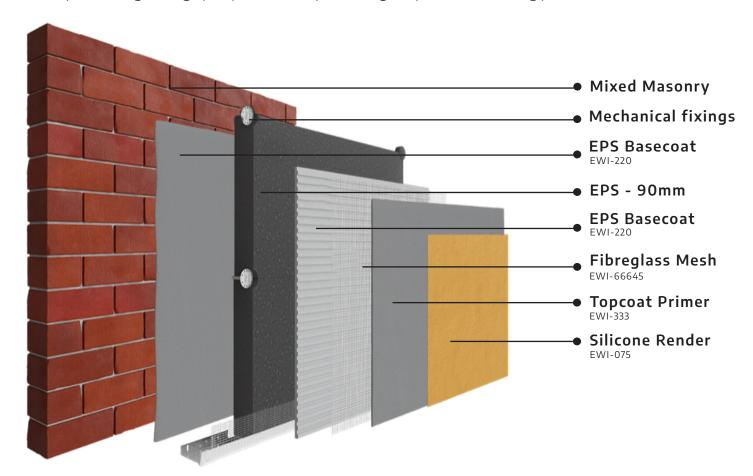
For this project, EPS insulation boards were used given their advanced thermal insulation properties, improving the substrate's U-Values. Coupled with a Silicone render, EPS also reduces the risk of water penetration and condensation. All the insulation boards in our external wall insulation systems are held in place by both an adhesive and mechanical fixings, so you can be sure that the system will remain for years to come.
