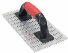
After allowing the first pass to begin curing but before it dries fully, the second coat of render should be applied at a thickness of 8mm. This will take the total thickness up to 17/18mm. After approximately 24 hours, once it has gone off, the render scratch float should be used to create the desired texture. The render should then be scratched back by 2mm. After rendering, the render will need a minimum of 48 hours to go off depending upon the weather.
